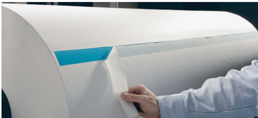
The protective liner should only be removed immediately before splicing.
