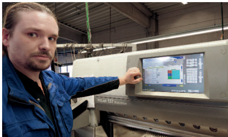
Cutter operator Michael Koller shows how the cutting programs are called up. The bar code scanner is located to the left on the cutter.
