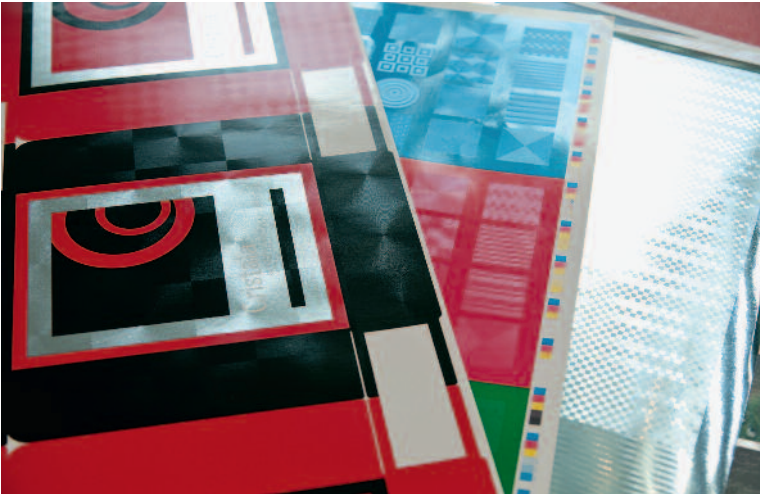
The Cristala project. The photographs show how existing drip-off equipment on offset presses can be used to produce new finishing effects. Specially prepared pre-press data allows the creation of structured surfaces with highly accentuated gloss.
