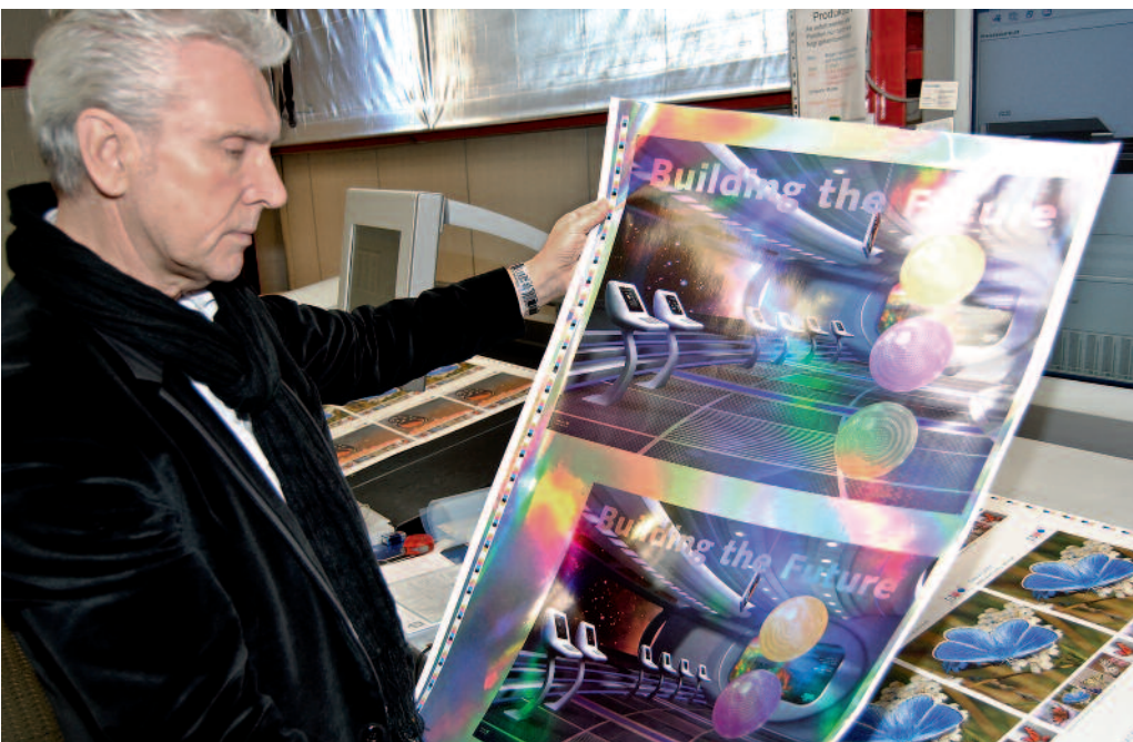
Multi-coating effects are a further print finishing variant, as shown here by the printing and finishing specialist Günter Thomas. They also highlight the latest holographic possibilities.
